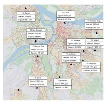
Figure 1. Heating plants and respective capacity in MW in Belgrade's DH.
